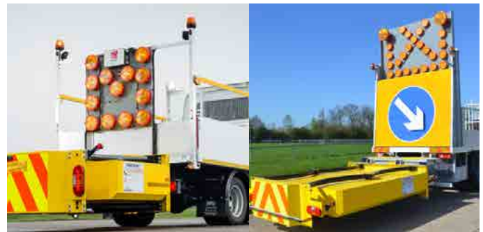
Pictures 2 and 3: Examples of vehicles fitted with impact protection used to alert other road Users of vehicles working from or immediately next to the road, provide appropriate information to drivers and to reduce the severity of injury should a road User collision with a works vehicle occur.
